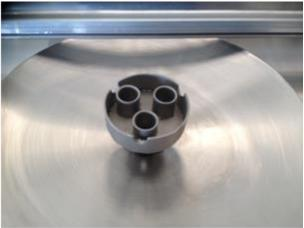
Nozzles are designed to be easily interchanged and can be positioned in any combination of X, Y or Z axis underneath the PCB with the aid of the PCB carrier. Control of solder wave height, alloy temperature and cycle time allow SOLDERWAVE to solder/desolder any PTH component.
